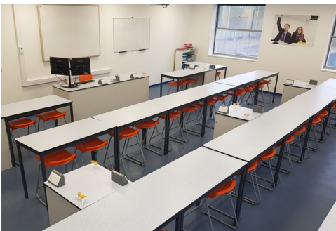
New lab with service bollards & Trespa work tops
